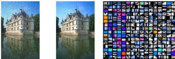
Figure: Left: input image; middle: denoised; right: dictionary for image patches.
