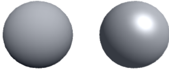
Figure 14.4 Comparison of a Lambertian (diffusive) sphere and a Phong (specular) sphere under the same (directional) lighting condition.
