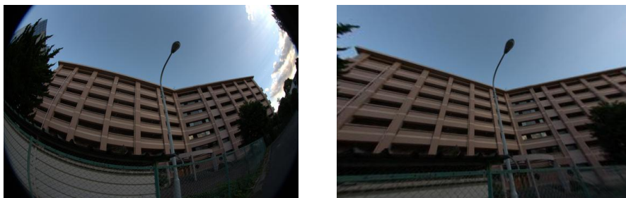
Figure 15.10 Left: typical image of a fisheye camera. Right: image of a perspective camera.
