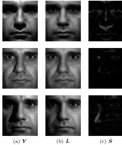
Figure 5.4 Removing shadows, specularities, and saturations from face images. (a) Cropped and aligned images of a person’s face under different illuminations from the Extended Yale Face Database B [GBK01]. The size of each image is 192 \times 168 pixels, a total of 58 different illuminations per person. (b) Low-rank approximation \hat{\mathbf{L}} recovered by convex programming. (c) Sparse error \hat{\mathbf{S}} corresponding to specularities in the eyes, shadows around the nose region, or brightness saturations on the face. Notice in the bottom left that the sparse term also compensates for errors in image acquisition.
